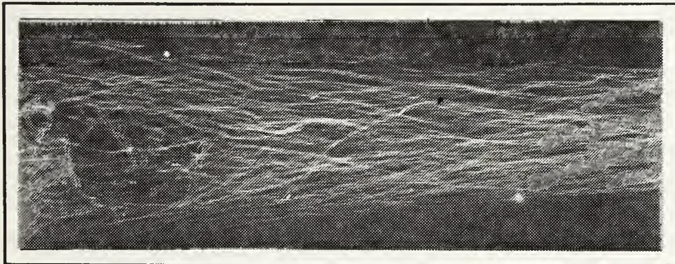
Figure 28. Typical Vortex Aft of Hangar - View from Vertical - 000^\circ yaw, 4^\circ pitch up, 5^\circ port roll.
